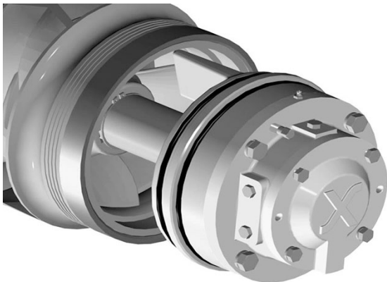
Figure 53: Bearing gland installed on bearing body
