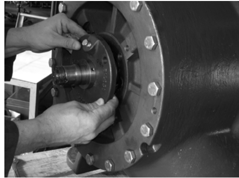
Figure 28: Removing the Gland Assembly and Sleeve
